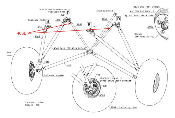
As a result of thorough investigation, it appeared that the parts broke due to a fatigue failure on one gusset of part number 405B of the main landing gear.
